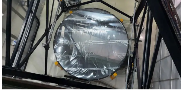
Figure 1: The image of the completed liquid mirror, covered in a thin mylar sheet to avoid contamination of the mercury. Credit: Aryabhata Research Institute of Observational Sciences (ARIES).
